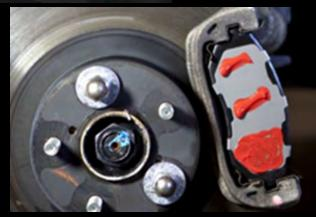
The use of anti squeal paste is also recommend when dealing with excessive brake pad movement, this helps hold brake pad stable within caliper bracket also caliper piston. However its very important once applied to brake system you allow enough curing time before road
