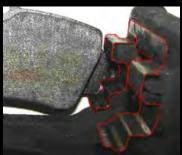
These improvements have been done for 1 reason only - to stop pad moving enough to reduce a torsional vibration that creates brake noise.
