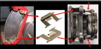
No 1. Mistake in fitting brake pads people don't clean & retention these spring clips and lubricate with high temp grease as it was done when vehicle was produced. New brake pads need to be tight in caliper brackets, that is the function of these spring clips.
